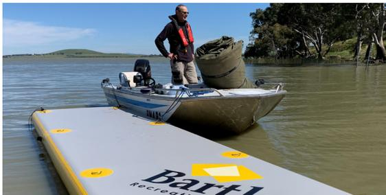
Built to last in Australian conditions, Bartlett Inflatable Pontoons are manufactured from commercial grade CE Certified Drop-Stitch Double Wall Fabric (DWF), designed to withstand a high amount of air pressure making them strong, rigid, and incredibly stable on the water. Most importantly, they are easy to deflate allowing to simply fit in a car or boat for transporting to and from the water.
