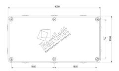
Created with D-rings top and bottom, the Bartlett 4Mx2M Deck Extender Pontoon has tie-points thoughtfully placed in positions that allow them to connect to other Bartlett Inflatable Pontoons across the range. Locking together other components such as the Bartlett Diamond Pontoon or Bartlett 8.5M Straight Pontoon allows endless possibilities for different shaped floating docks accommodating so many situations.
