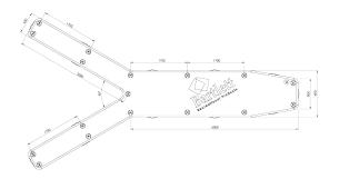
Created with D-rings top and bottom, the Bartlett 8.5M Y Pontoon has tie-points thoughtfully placed in positions that allow connection to other Bartlett Inflatable Pontoons across the range. Locking together other components such as the Bartlett Diamond Pontoon or Bartlett 4Mx2M Deck Extender Pontoon allows endless possibilities for different shaped floating docks accommodating so many situations.
