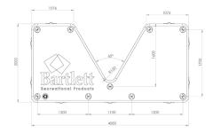
Created with D-rings top and bottom, the Bartlett 4Mx2M V Deck Pontoon has tie-points thoughtfully placed in positions that allow them to connect to other Bartlett Inflatable Pontoons across the range. Locking together other components such as the Bartlett 8.5M Straight Pontoon allows endless possibilities for different shaped floating docks accommodating so many situations.
